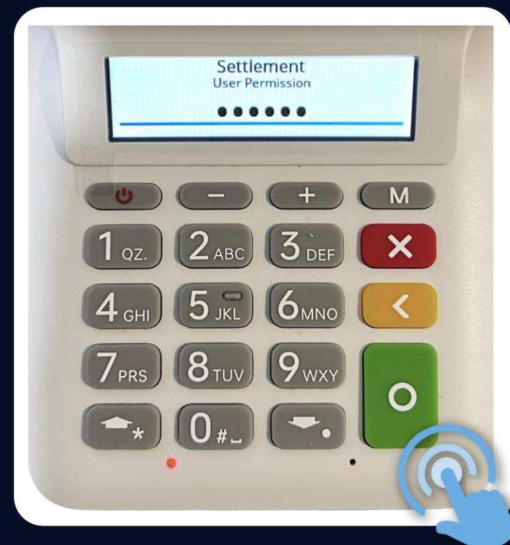
**STEP 2** Key in **Settlement Password** (Last 6 digits of TID) and press **Enter**
